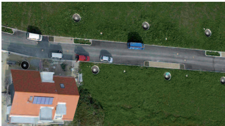
Aerial view showing 'Innodrain' percolation beds with subterranean French drain in the street area, and a 'Terra' rainwater tank with earth filter on every lot.
